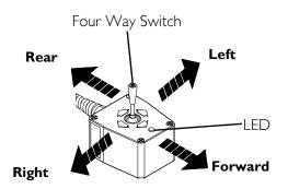
FIGURE 5.1 Using the Four Way Switch
